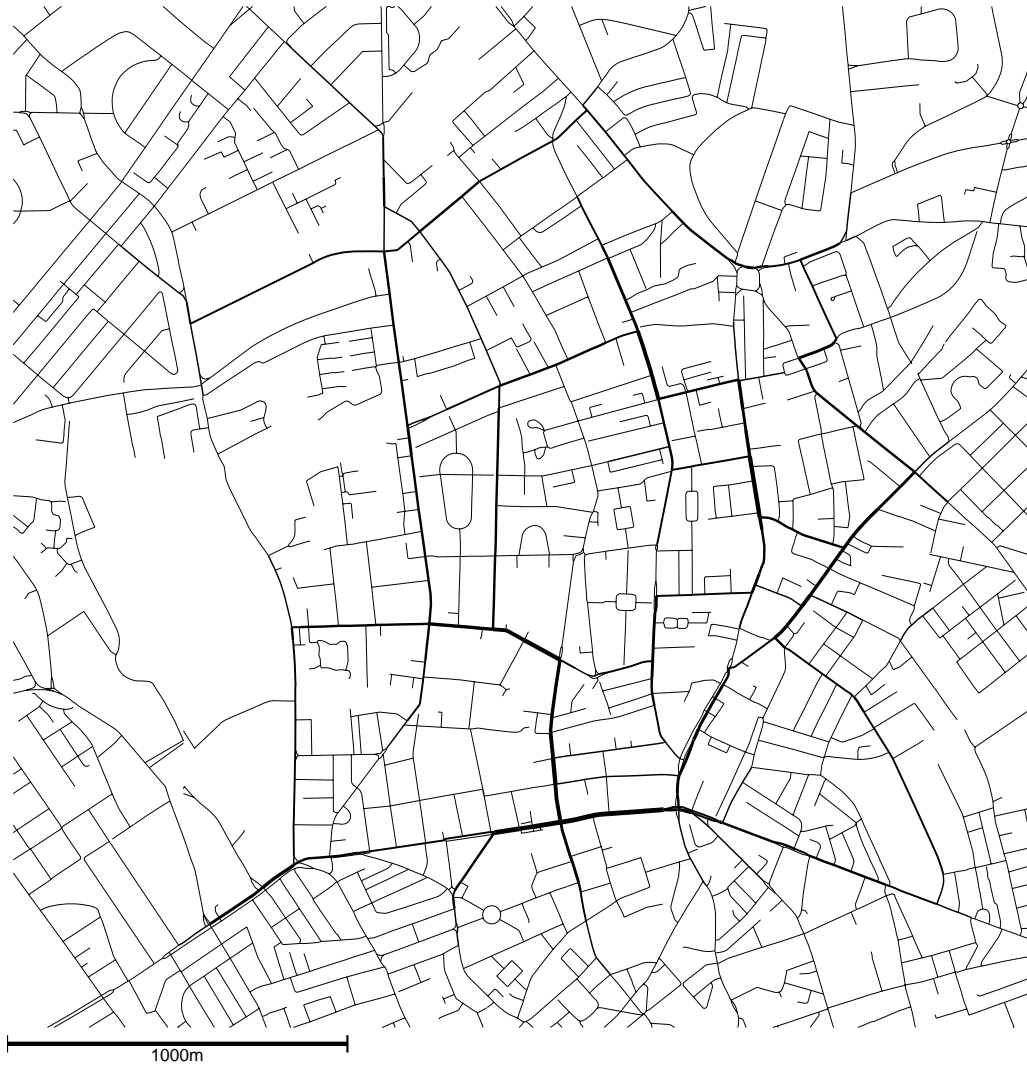
Figure 58: Weighted choice for a 3\text{km} \times 3\text{km} system of road-centre lines. Thicker lines have higher values.
