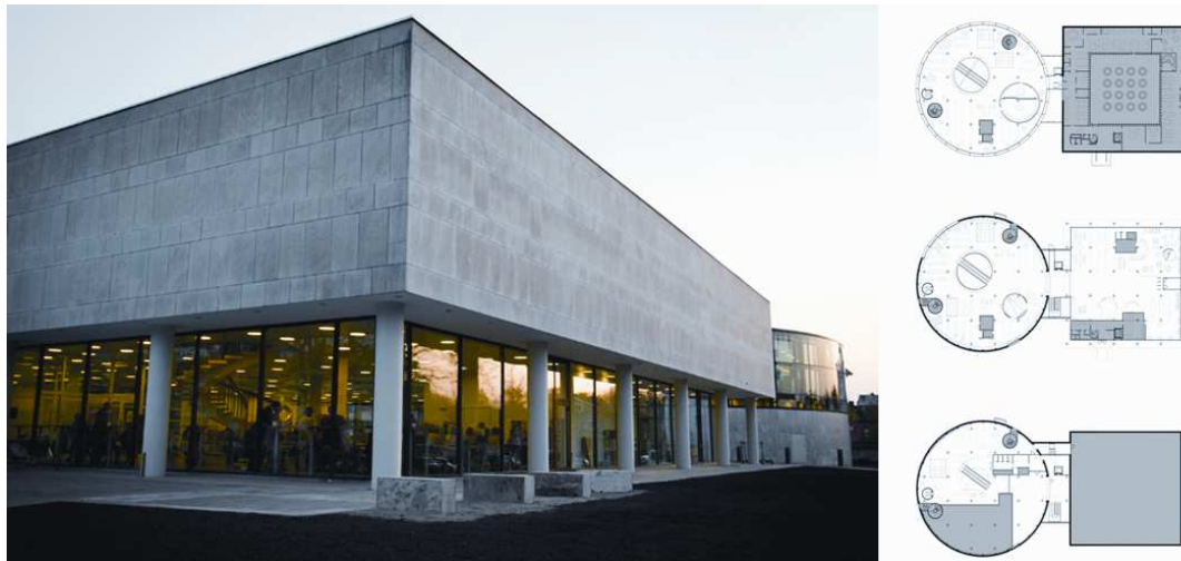
Figure - The City Library of Växjö - exterior photography and plans, presented in ascending order from the bottom up, entrance on middle floor. Greyed areas are not accessible by the public.
