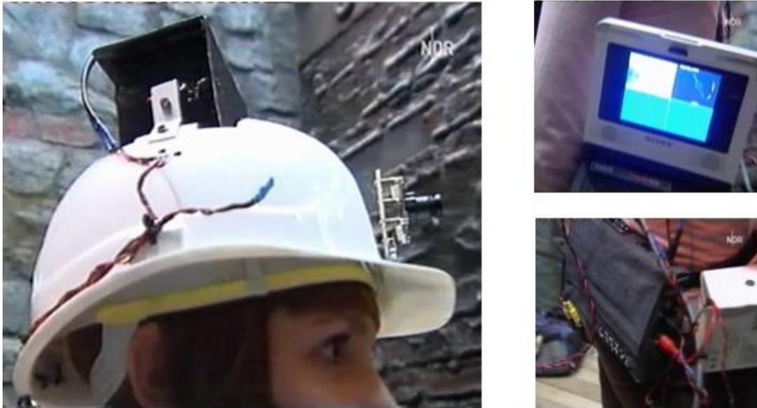
*Figure 2:* Equipment for the recording of movement and orientation behaviour (compass and second camera are mounted in the black box).
